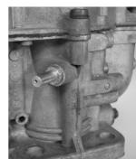
4-mm hole, and cutting M5-thread into the dual choke carburettor (see photo) because these are already prepared for a vacuum nipple. The nipple is supplied with the 123\EVO.
